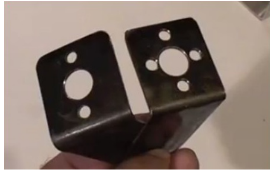
Figure 3.11: Front of the L-shape motor mount
