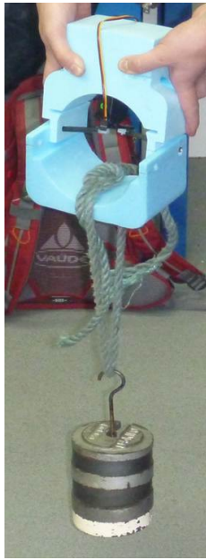
Figure 5.12: Foam tear and pin deflection test setup
