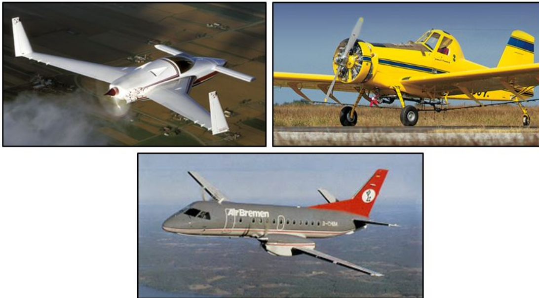
Figure 3.5: Engine Configurations: Pusher(top-left)[39], Tractor(top-right)[21] and Wing Mounted(bottom)[125]
