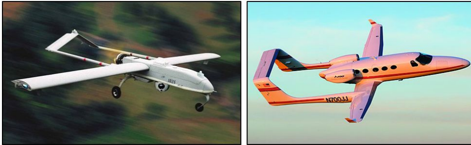
Figure 3.4: Inverted V-Tail [14] (Left) and Twin Boom T-Tail [86](Right)
